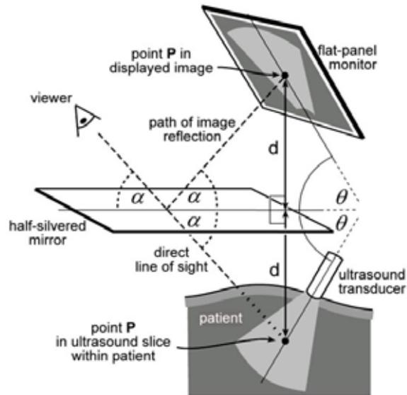
Fig. 2.1. Optics of Real-Time Tomographic Reflection (RTTR) in the Sonic Flashlight
