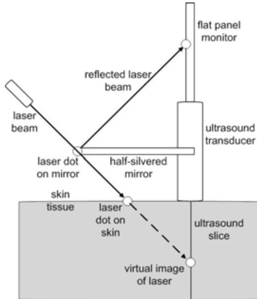
**Fig. 3.1.** Laser Needle Guide optics overview (see text).
