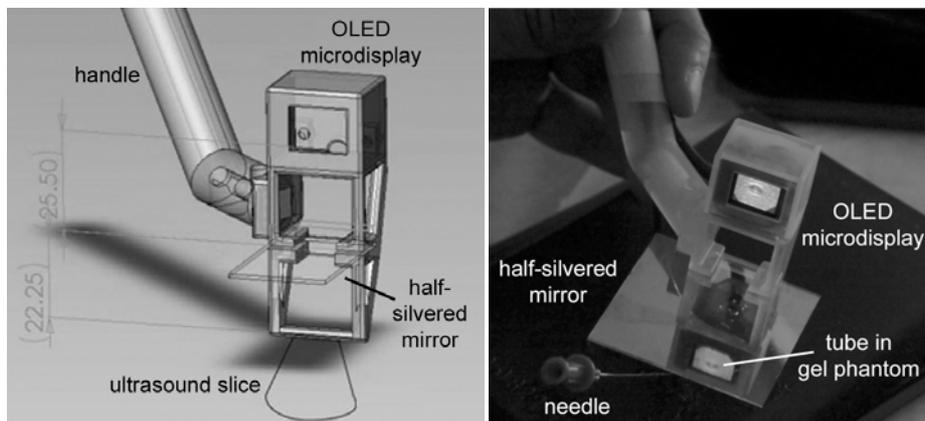
**Fig. 1.** Left: CAD/CAM design of the Sonic Penlight housing. Right: First prototype of the Sonic Penlight and the insertion of needle into a gel phantom with its guidance.
